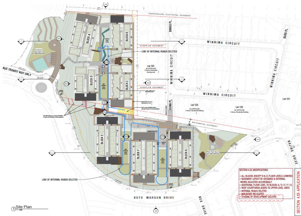
Figure 5 - Site Plan showing proposed deletion of internal roads dashed in blue (Drawing No. S01, Issue I, prepared by Architex, dated 14/05/2021)
